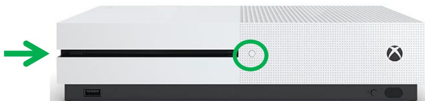
Figure 16. An Xbox One S console, highlighting the disc tray (arrow) and eject button (circle)
